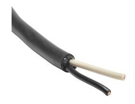
Southwire portable cord, unshielded, SJOOW, 300V, 2 conductors, 14 AWG, EPDM thermoset rubber conductor insulation material, black and white, CPE thermoset rubber jacket, black, cut to length.
