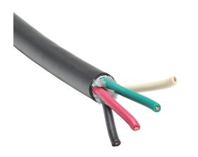
Southwire portable cord, unshielded, SJOOW, 300V, 4 conductors (includes ground), 12 AWG, EPDM thermoset rubber conductor insulation material, black, white, red and green, CPE thermoset rubber jacket, black, cut to length.
