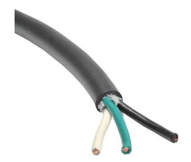
Southwire portable cord, unshielded, SJOOW, 300V, 3 conductors (includes ground), 12 AWG, EPDM thermoset rubber conductor insulation material, black, white and green, CPE thermoset rubber jacket, black, cut to length.
