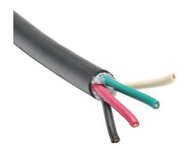
Southwire portable cord, unshielded, SJOOW, 300V, 4 conductors (includes ground), 10 AWG, EPDM thermoset rubber conductor insulation material, black, white, red and green, CPE thermoset rubber jacket, black, cut to length.
