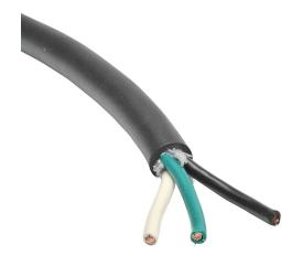
Southwire portable cord, unshielded, SJOOW, 300V, 3 conductors (includes ground), 10 AWG, EPDM thermoset rubber conductor insulation material, black, white and green, CPE thermoset rubber jacket, black, cut to length.
