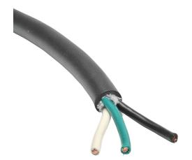
Southwire portable cord, unshielded, SJOOW, 300V, 3 conductors (includes ground), 10 AWG, EPDM thermoset rubber conductor insulation material, black, white and green, CPE thermoset rubber jacket, black, cut to length.
