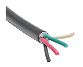
Southwire portable cord, unshielded, SJEOOW, 300V, 4 conductors (includes ground), 18 AWG, TPE conductor insulation material, black, white, red and green, TPE jacket, black, cut to length.
