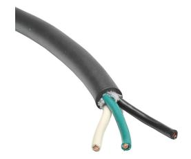
Southwire portable cord, unshielded, SJEOOW, 300V, 3 conductors (includes ground), 18 AWG, TPE conductor insulation material, black, white and green, TPE jacket, black, cut to length.
