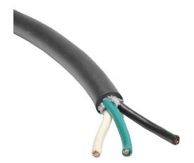
Southwire portable cord, unshielded, SJEOOW, 300V, 3 conductors (includes ground), 18 AWG, TPE conductor insulation material, black, white and green, TPE jacket, black, cut to length.
