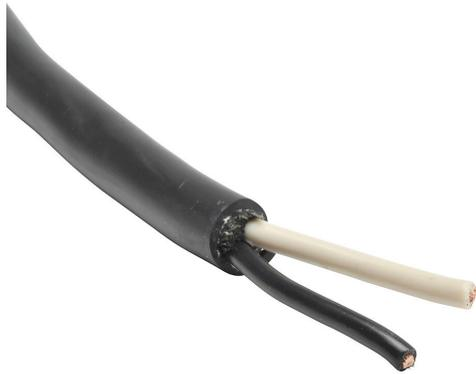
Southwire portable cord, unshielded, SJEOOW, 300V, 2 conductors, 18 AWG, TPE conductor insulation material, black and white, TPE jacket, black, cut to length.
