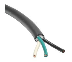
Southwire portable cord, unshielded, SJEOOW, 300V, 3 conductors (includes ground), 16 AWG, TPE conductor insulation material, black, white and green, TPE jacket, black, cut to length.
