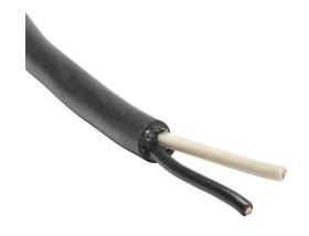
Southwire portable cord, unshielded, SJEOOW, 300V, 2 conductors, 16 AWG, TPE conductor insulation material, black and white, TPE jacket, black, cut to length.
