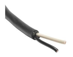
Southwire portable cord, unshielded, SJEOOW, 300V, 2 conductors, 14 AWG, TPE conductor insulation material, black and white, TPE jacket, black, cut to length.
