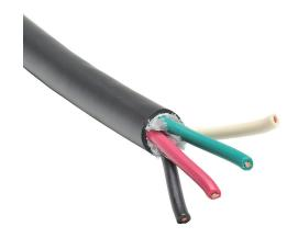
Southwire portable cord, unshielded, SJEOOW, 300V, 4 conductors (includes ground), 12 AWG, TPE conductor insulation material, black, white, red and green, TPE jacket, black, cut to length.
