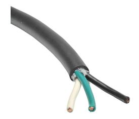
Southwire portable cord, unshielded, SJEOOW, 300V, 3 conductors (includes ground), 12 AWG, TPE conductor insulation material, black, white and green, TPE jacket, black, cut to length.
