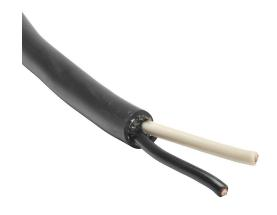
Southwire portable cord, unshielded, SJEOOW, 300V, 2 conductors, 12 AWG, TPE conductor insulation material, black and white, TPE jacket, black, cut to length.
