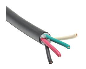
Southwire portable cord, unshielded, SJEOOW, 300V, 4 conductors (includes ground), 10 AWG, TPE conductor insulation material, black, white, red and green, TPE jacket, black, cut to length.
