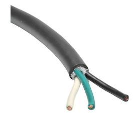
Southwire portable cord, unshielded, SJEOOW, 300V, 3 conductors (includes ground), 10 AWG, TPE conductor insulation material, black, white and green, TPE jacket, black, cut to length.
