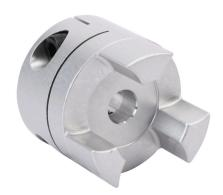
Sung-II Machinery drive coupling hub, jaw type, aluminum alloy, clamp, size 40, 3/8in bore. Requires SJC-40 series spiders.
