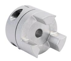
Sung-II Machinery drive coupling hub, jaw type, aluminum alloy, clamp, size 40, 8mm bore. Requires SJC-40 series spiders.
