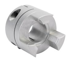
Sung-II Machinery drive coupling hub, jaw type, aluminum alloy, clamp, size 40, 19mm bore. Requires SJC-40 series spiders.
