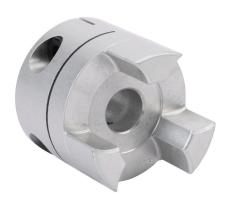
Sung-II Machinery drive coupling hub, jaw type, aluminum alloy, clamp, size 40, 12mm bore. Requires SJC-40 series spiders.
