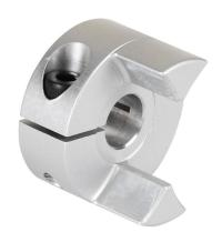
Sung-II Machinery drive coupling hub, jaw type, aluminum alloy, clamp, size 30, 3/8in bore. Requires SJC-30 series spiders.
