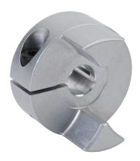
Sung-II Machinery drive coupling hub, jaw type, aluminum alloy, clamp, size 30, 5/16in bore. Requires SJC-30 series spiders.
