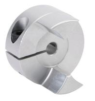
Sung-II Machinery drive coupling hub, jaw type, aluminum alloy, clamp, size 30, 5mm bore. Requires SJC-30 series spiders.
