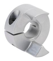
Sung-II Machinery drive coupling hub, jaw type, aluminum alloy, clamp, size 30, 12mm bore. Requires SJC-30 series spiders.
