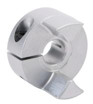
Sung-II Machinery drive coupling hub, jaw type, aluminum alloy, clamp, size 30, 10mm bore. Requires SJC-30 series spiders.
