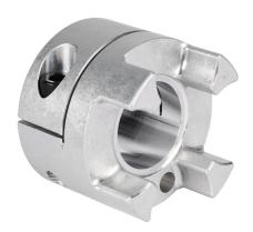
Sung-II Machinery drive coupling hub, jaw type, aluminum alloy, clamp, size 80, 40mm bore. Requires SJC-80 series spiders.
