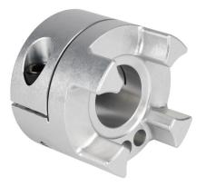
Sung-II Machinery drive coupling hub, jaw type, aluminum alloy, clamp, size 80, 35mm bore. Requires SJC-80 series spiders.
