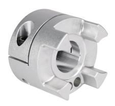
Sung-II Machinery drive coupling hub, jaw type, aluminum alloy, clamp, size 80, 32mm bore. Requires SJC-80 series spiders.
