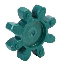
Sung-II Machinery drive coupling spider, jaw type, size 80, Hytrel, 98A durometer. For use with SJC-80C series hubs.
