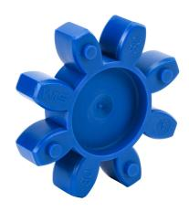
Sung-II Machinery drive coupling spider, jaw type, size 80, thermoplastic polyurethane, 98A durometer. For use with SJC-80C series hubs.
