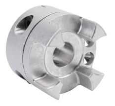
Sung-II Machinery drive coupling hub, jaw type, aluminum alloy, clamp, size 65, 20mm bore. Requires SJC-65 series spiders.
