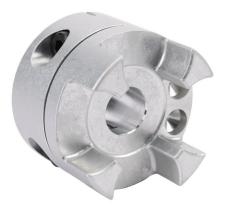
Sung-II Machinery drive coupling hub, jaw type, aluminum alloy, clamp, size 65, 3/4in bore. Requires SJC-65 series spiders.
