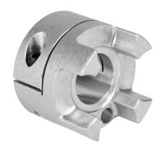
Sung-II Machinery drive coupling hub, jaw type, aluminum alloy, clamp, size 55, 1in bore. Requires SJC-55 series spiders.
