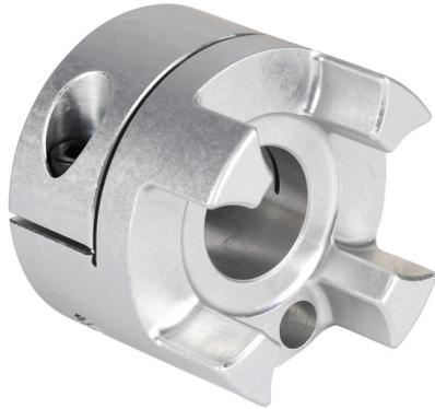
Sung-II Machinery drive coupling hub, jaw type, aluminum alloy, clamp, size 55, 22mm bore. Requires SJC-55 series spiders.
