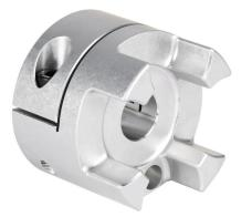
Sung-Il Machinery drive coupling hub, jaw type, aluminum alloy, clamp, size 55, 5/8in bore. Requires SJC-55 series spiders.
