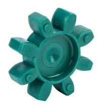
Sung-II Machinery drive coupling spider, jaw type, size 55, Hytrel, 98A durometer. For use with SJC-55C series hubs.
