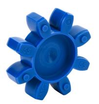
Sung-II Machinery drive coupling spider, jaw type, size 55, thermoplastic polyurethane, 98A durometer. For use with SJC-55C series hubs.
