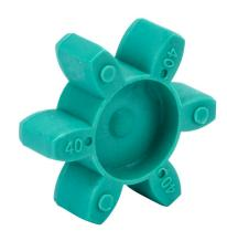
Sung-II Machinery drive coupling spider, jaw type, size 40, Hytrel, 98A durometer. For use with SJCB-40C series hubs.
