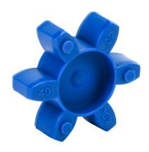
Sung-II Machinery drive coupling spider, jaw type, size 40, thermoplastic polyurethane, 98A durometer. For use with SJCB-40C series hubs.
