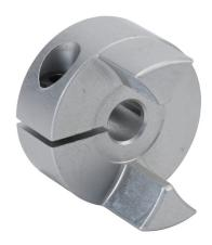
Sung-II Machinery drive coupling hub, jaw type, aluminum alloy, clamp, size 25, 6mm bore. Requires SJC-25 series spiders.
