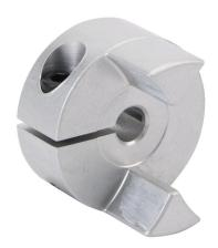
Sung-II Machinery drive coupling hub, jaw type, aluminum alloy, clamp, size 25, 5mm bore. Requires SJC-25 series spiders.
