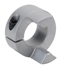
Sung-II Machinery drive coupling hub, jaw type, aluminum alloy, clamp, size 25, 14mm bore. Requires SJC-25 series spiders.
