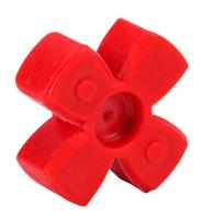
Sung-II Machinery drive coupling spider, jaw type, size 25, Hytrel, 63D durometer. For use with SJC-25C series hubs.
