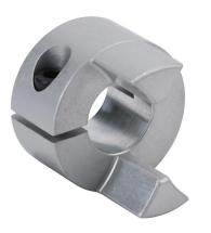
Sung-II Machinery drive coupling hub, jaw type, aluminum alloy, clamp, size 20, 3/8in bore. Requires SJC-20 series spiders.
