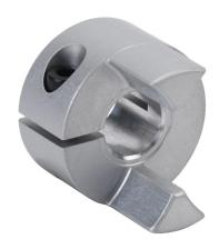
Sung-II Machinery drive coupling hub, jaw type, aluminum alloy, clamp, size 20, 5/16in bore. Requires SJC-20 series spiders.
