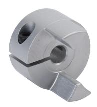
Sung-II Machinery drive coupling hub, jaw type, aluminum alloy, clamp, size 20, 5mm bore. Requires SJC-20 series spiders.
