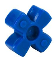
Sung-II Machinery drive coupling spider, jaw type, size 20, thermoplastic polyurethane, 98A durometer. For use with SJC-20C series hubs.
