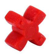
Sung-II Machinery drive coupling spider, jaw type, size 14, Hytrel, 63D durometer. For use with SJC-14C series hubs.
