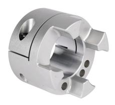
Sung-II Machinery drive coupling hub, jaw type, aluminum alloy, clamp, size 100, 60mm bore. Requires SJC-100 series spiders.
