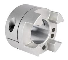
Sung-II Machinery drive coupling hub, jaw type, aluminum alloy, clamp, size 100, 55mm bore. Requires SJC-100 series spiders.
